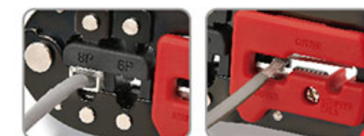
Build-in crimp dies for 6P/8P modular connector
