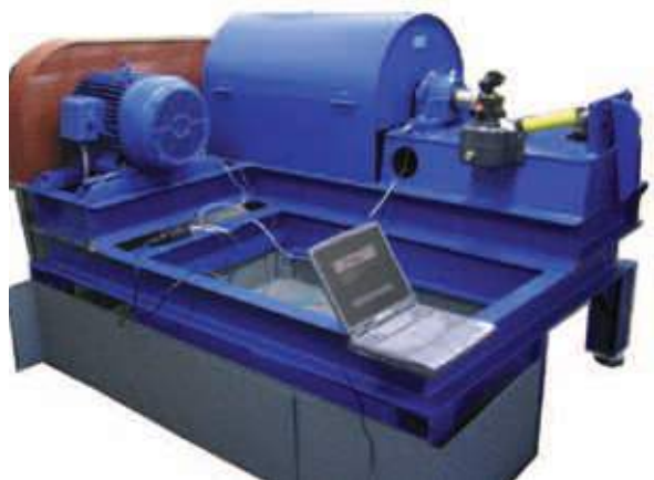
Housing and seals on the test bench. Vibration behaviour, temperature pattern and wear behaviour in practice.
