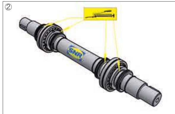
② Clamp the shaft horizontally (protect the shaft against damage in the area of the clamping). Slide the internal labyrinth rings onto the shaft. Ensure the correct mounting direction. On units with an internal shaft end, only one labyrinth seal is used. The cover plate SC..EC is used instead of the second seal in this case. The bearings should be positioned on the shaft as described in the Mounting the bearings section and completely filled with grease. Then position the external labyrinth rings on the shaft in the correct mounting direction.
