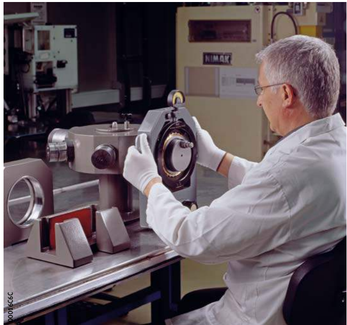
Figure 4 Positioning the enveloping circle gauge
