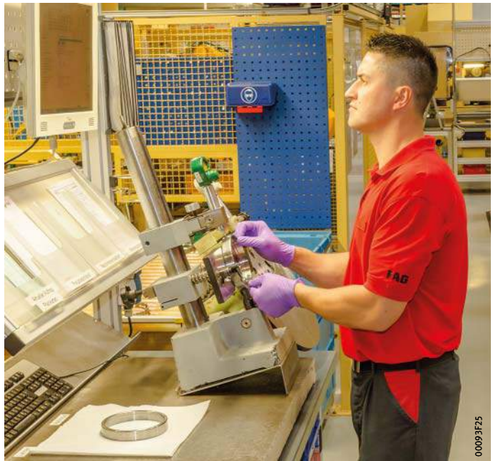
Figure 2 ... in the mounting of bearings
