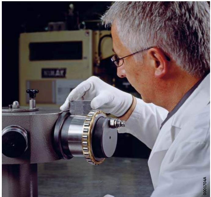
Figure 5 Measuring the spacing from the shaft shoulder
