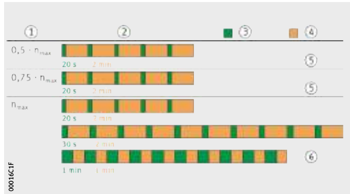
Figure 4 Grease distribution cycle for open and sealed spindle bearings
